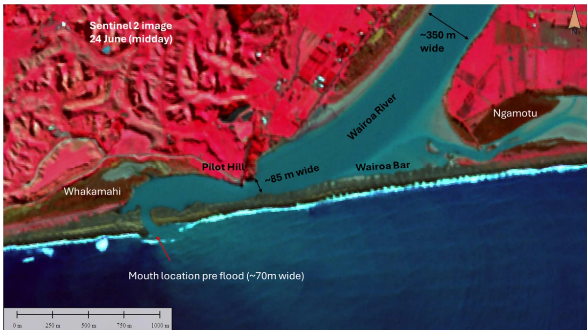
Figure 2.10: Annotated satellite image showing the bar position two days before the flooding event. Source: https://browser.dataspace.copernicus.eu/
