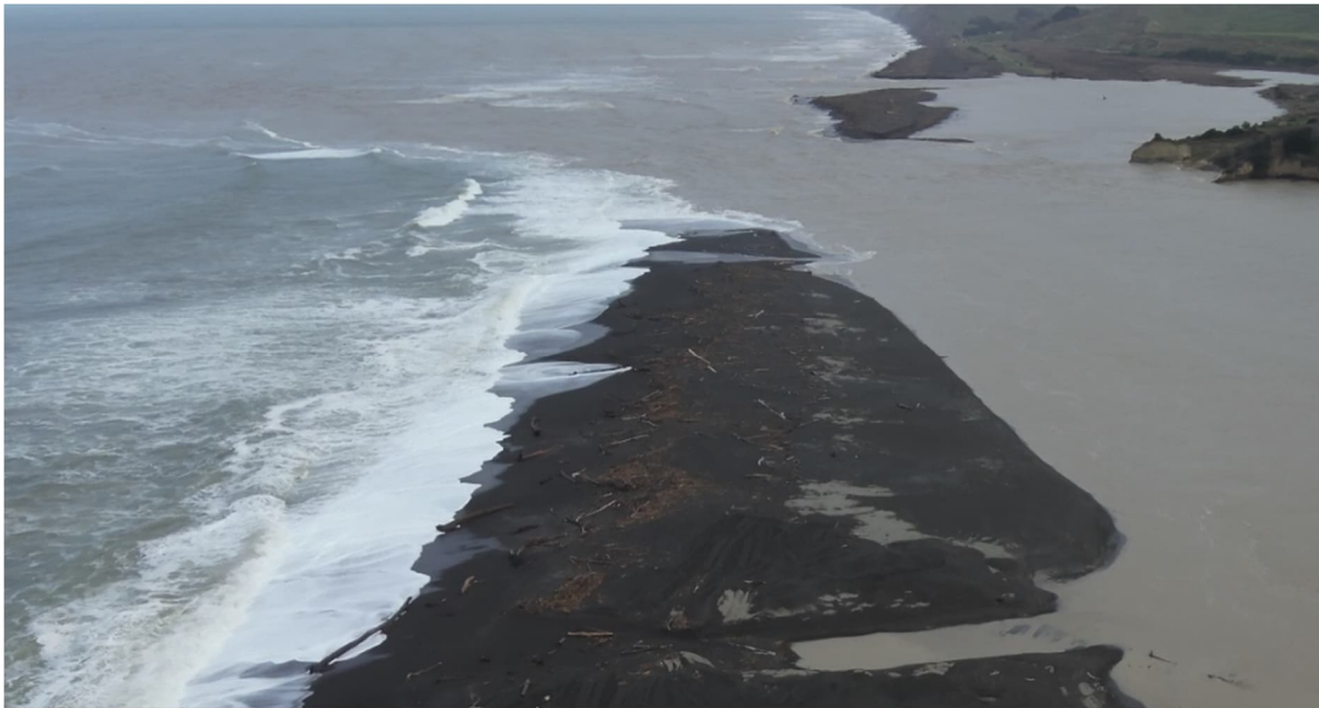
Figure 5.12: Snapshot from a UAV video provided by HBRC the day after the flood event showing an area of no surf-zone aligned with the outflowing.
