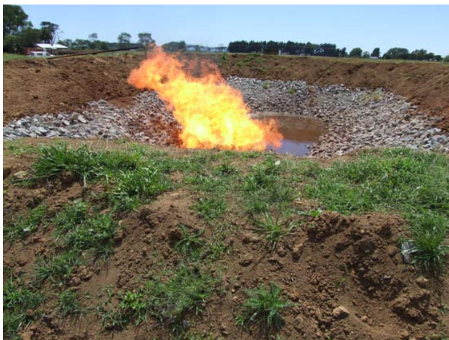
Figure 13: Lined flare pit with hydrocarbons being flared (Source: Taranaki Regional Council)
