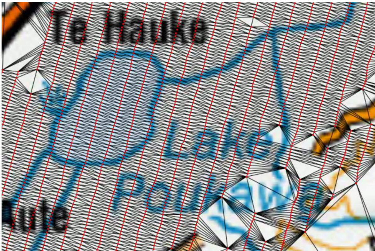
Figure 4.3 Example set-up of spatially constrained inversion constraints. The red points are the model positions. The black lines show the constraints created with the Delaunay triangles. The line distance in this example is 200 m.
