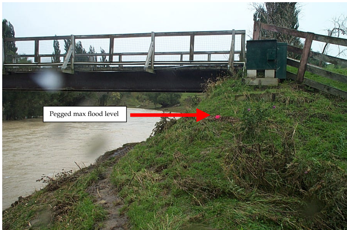
Figure 5: Mangaorapa Water Level Recorder with pegged maximum flood level.
