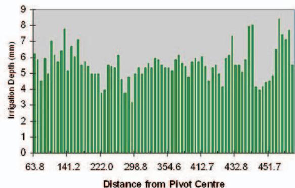
*Figure 1. Graph illustrating the distribution uniformity along the length of the centre pivot.  $DUIq = 0.77$*
