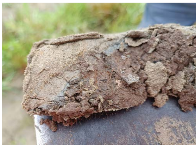
Example of differential deposition across topsoil– perfect for incorporation. Silt Layer is <20cm, blue/grey layer caused by lack of oxygen and both fine and coarse sand visible. A shallow rip and cultivation will aerate and address shallow deposition.
