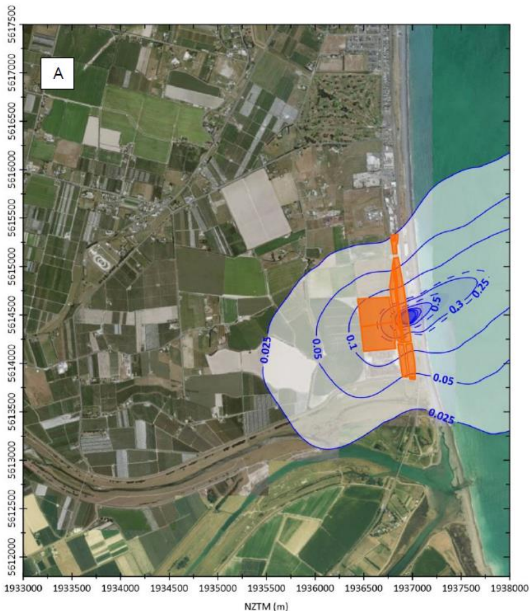
Figure 1. Modelled 90-day average atmospheric fluoride (F) concentrations ( \mu\text{g}/\text{m}^3 ) at ground level around the Napier Works for the existing stack scenario. Ravensdown-owned land is shaded orange. The model assumed the Napier Works was emitting F at the 75th percentile of measured manufacturing rates. Source: Chilton (2021).
