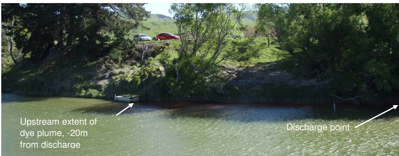
Figure 17 – Rhodamine Dye plume on outgoing tide, -20m to 0m from discharge point. Taken at 10:50, 1hr after high tide, 20min after release of dye.
