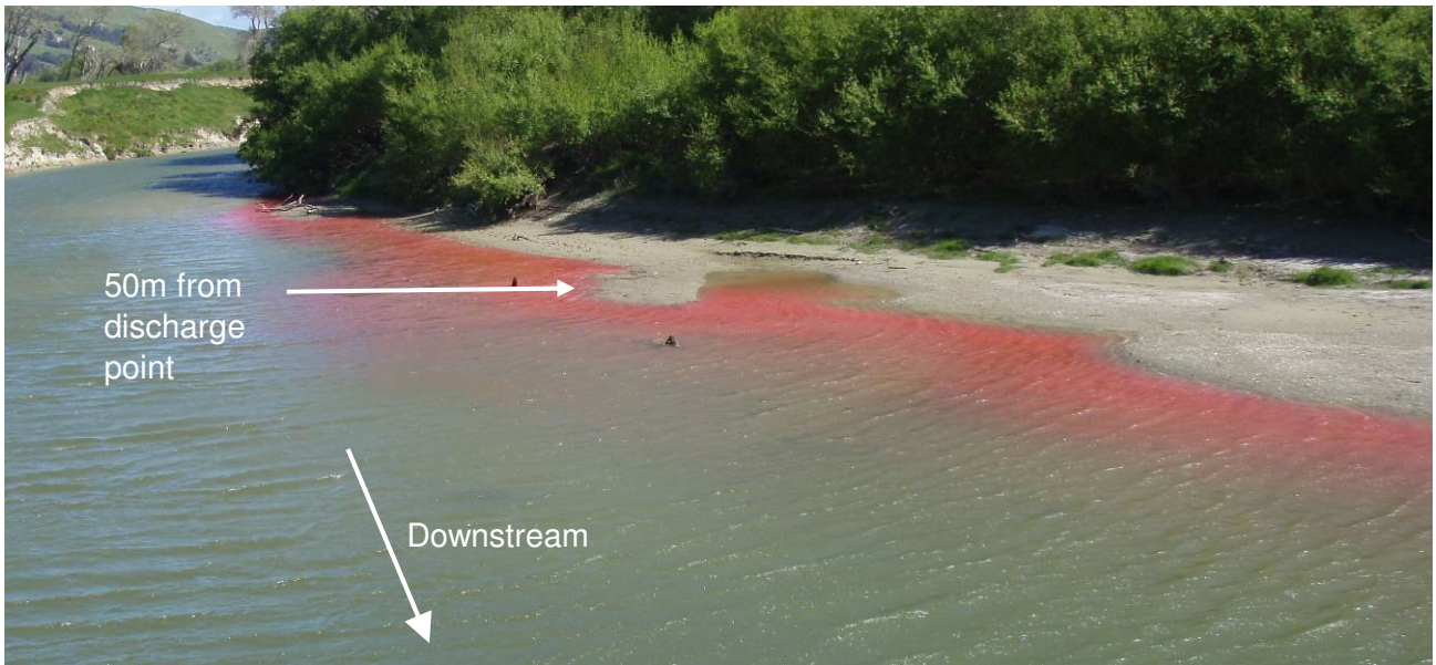
Figure 18 - Rhodamine dye plume on outgoing tide, 0 to 100m from discharge point. Taken at 11:30, 1hr 40min after high tide, 1hr after release of dye.
