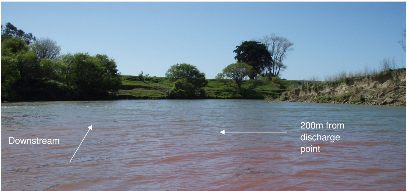
Figure 20 - Rhodamine dye plume on outgoing tide, 150 to 300m from discharge point.
