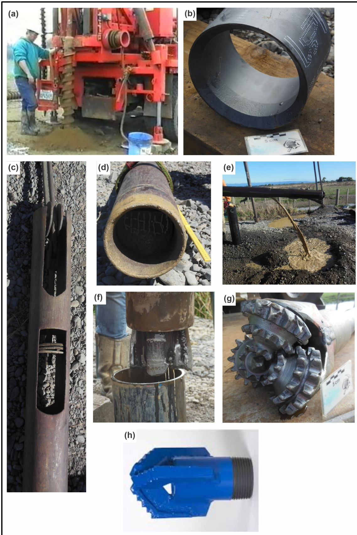
Figure 2.3 Examples of drilling equipment: (a) auger drilling; (b) hardened drive shoe; (c) upper section of a cable tool bailer, showing piston; (d) bottom of cable tool bailer; (e) emptying cable tool bailer; (f) chisel being withdrawn from the top of the casing; (g) tricone rotary bit; (h) rotary drag bit.
