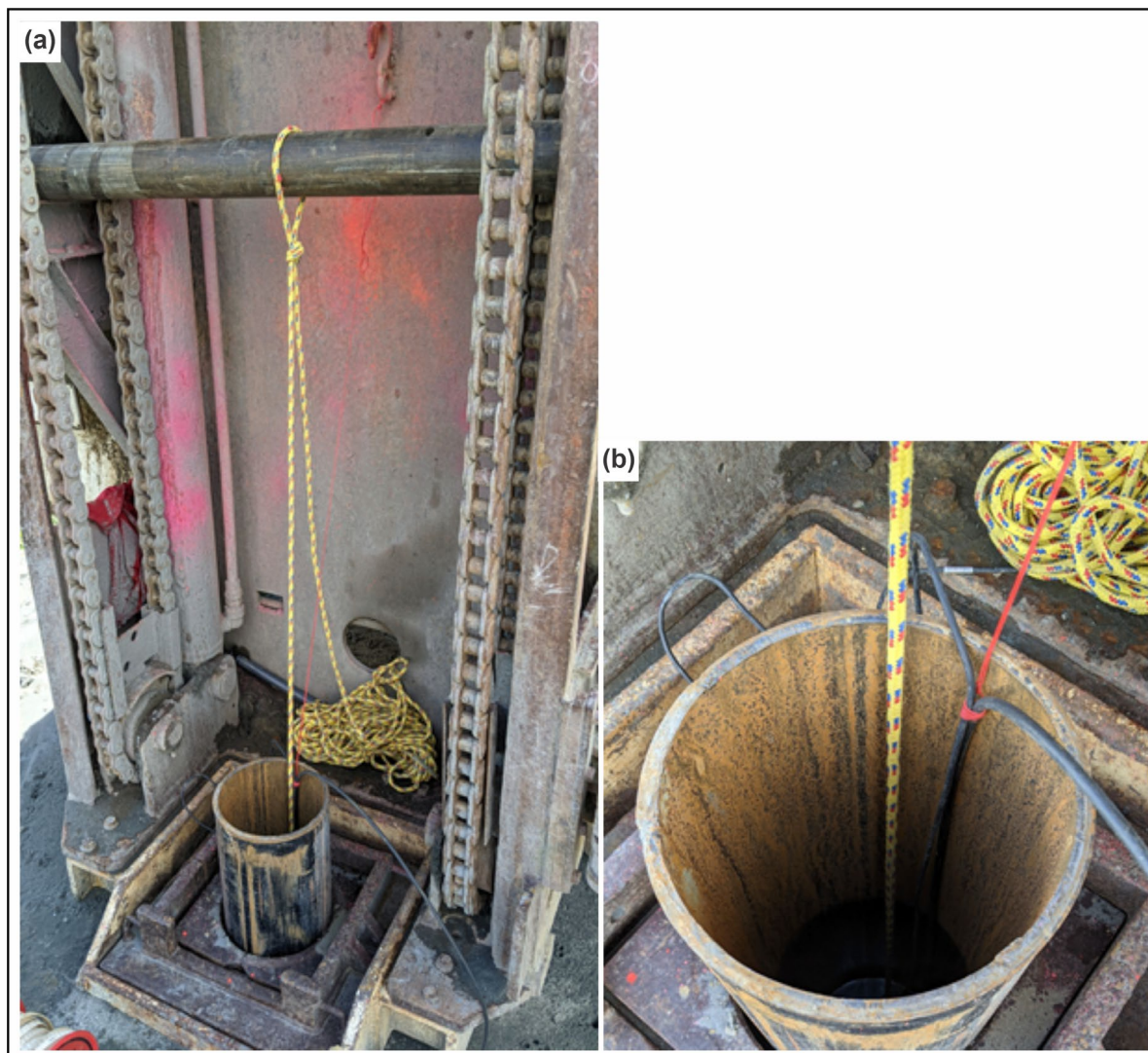
Figure 2.10 Picture of the slug test settings: (a) the yellow cord holding the slug and the red cord holding the two data loggers' cables were attached to a fixed part of the rig; (b) close-up picture of the red and yellow cords.
