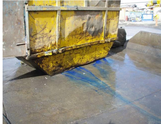
Example of a Waste Bin Leaking Paint into the Stormwater Drainage System
