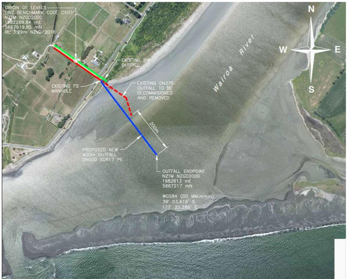
**Figure 4. Proposed replacement outfall pipeline structure location (blue) and relocation area (yellow) with the existing outfall structure in red**
