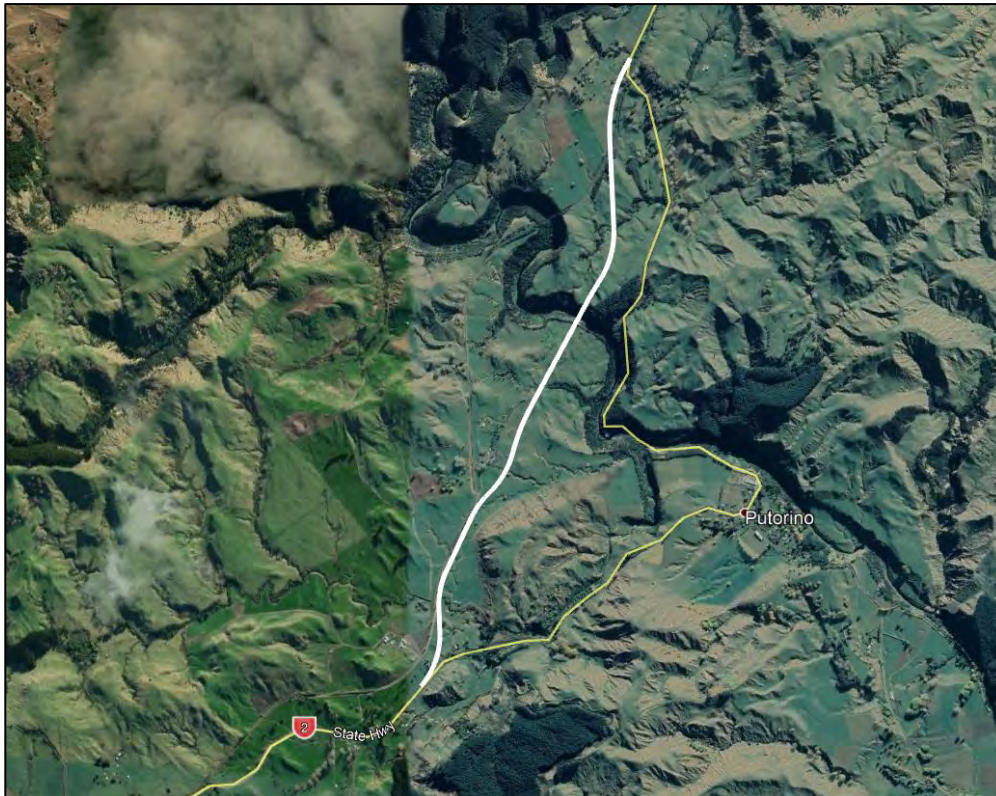
Figure 1: The proposed route of the realigned SH2 (white line). The present alignment is shown in yellow.
