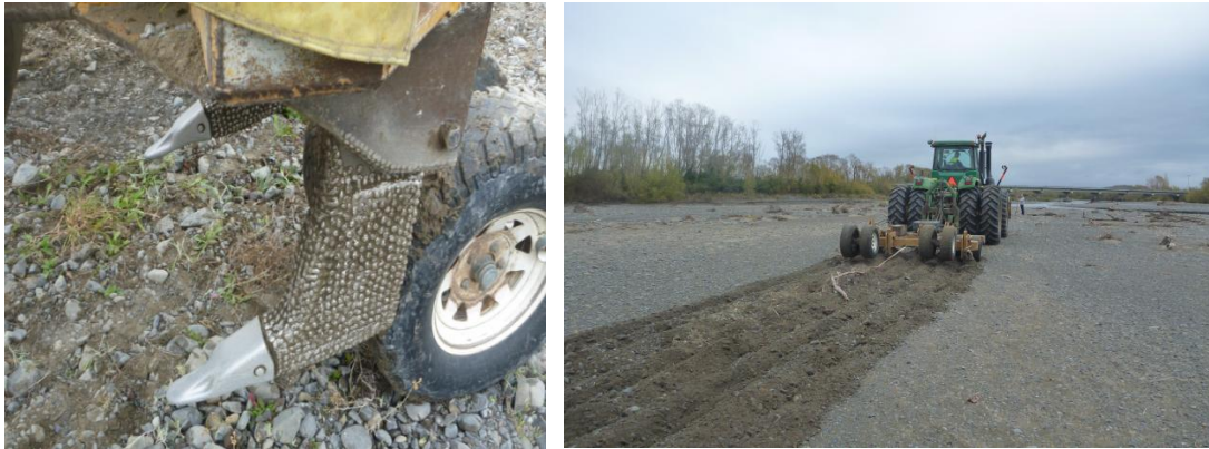
Figure 2. Gravel bar ripper tractor trailer assembly (figure reproduced from Warman 2013).
