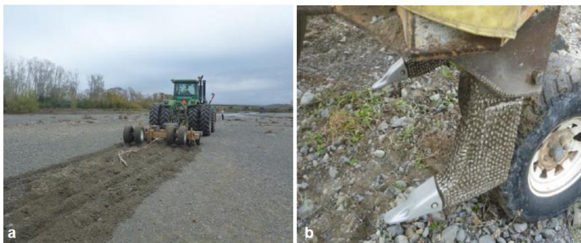
Figure 2-3: River gravel beach raking (a) in the Waipawa River in Hawke's Bay and (b) a close-up view of the large metal ripping blades on the tractor and trailer unit. Rippers designed by G Clode.
