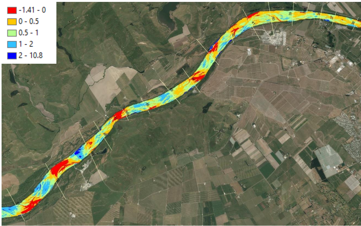
Figure 2-14 Ngaruroro River XS 36 to XS 51 showing bed levels relative to the grade line. Red areas represent locations where gravel extraction is not currently permitted. The image readily shows areas of aggradation and degradation to provide a visual guide to extraction locations.
