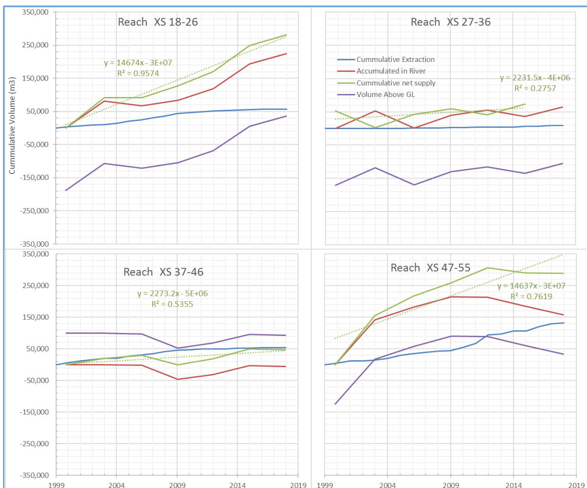
Figure 8-21: Cumulative volume analysis for different reaches in the Tutaekuri River
