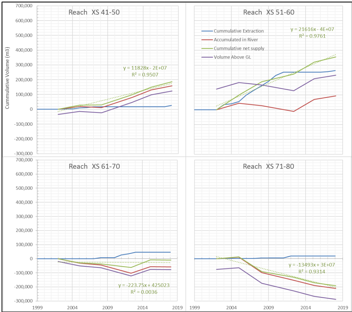
Figure 9-22: Cumulative volume analysis for different reaches between XS 41 and XS 80 in the Upper Tukituki River
