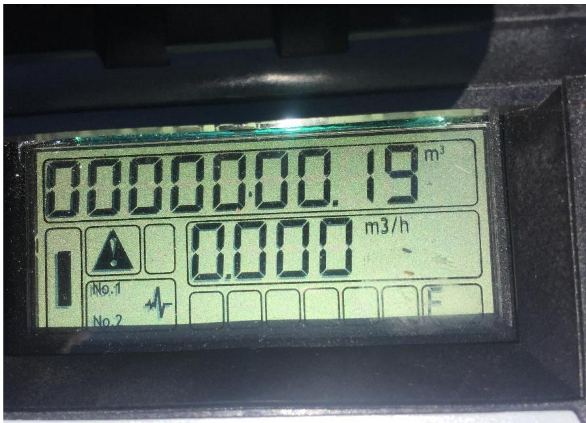
The top line is the cumulative volume. This meter has had 0.19m<sup>3</sup> pass through it or 190Litres (new installation)
