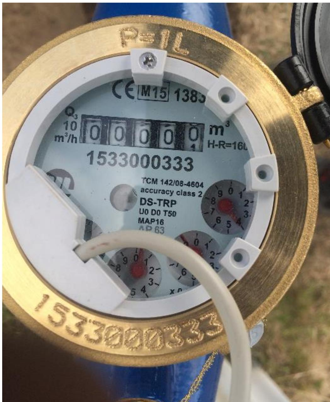
Like the first meter the top dial in black is displaying whole cubes and the red arrowed dials are the decimals. This meter could be confused with a meter where the top dial is reporting in 10's of cubic meters due to the Q3  $10\text{m}^3/\text{hr}$  which is on the left hand side. This actually is saying the maximum quantity the meter can record and report accurately is  $10\text{m}^3/\text{hr}$  or a maximum flow rate of 2.77litres/second.
