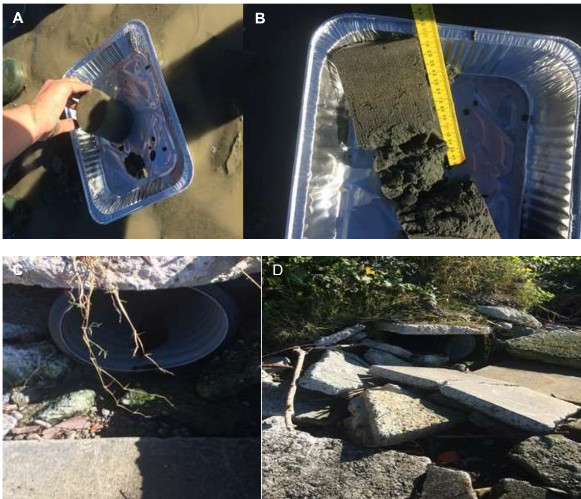
Figure 2 A) Replicate sediment core; B) sediment core split in half to evaluate RDL layer; C) and D) overflow adjacent Kopu Rd/Fitzroy St intersection.
