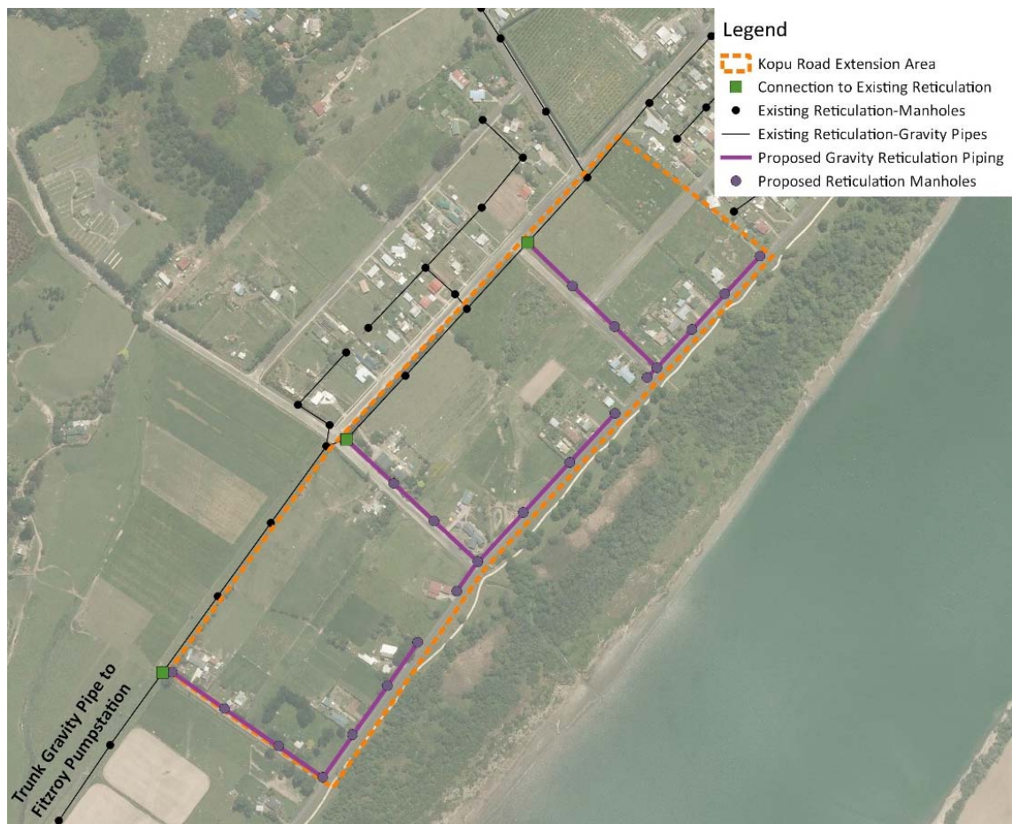
Figure 4.15 Kopu Road Extension Area - Gravity System
