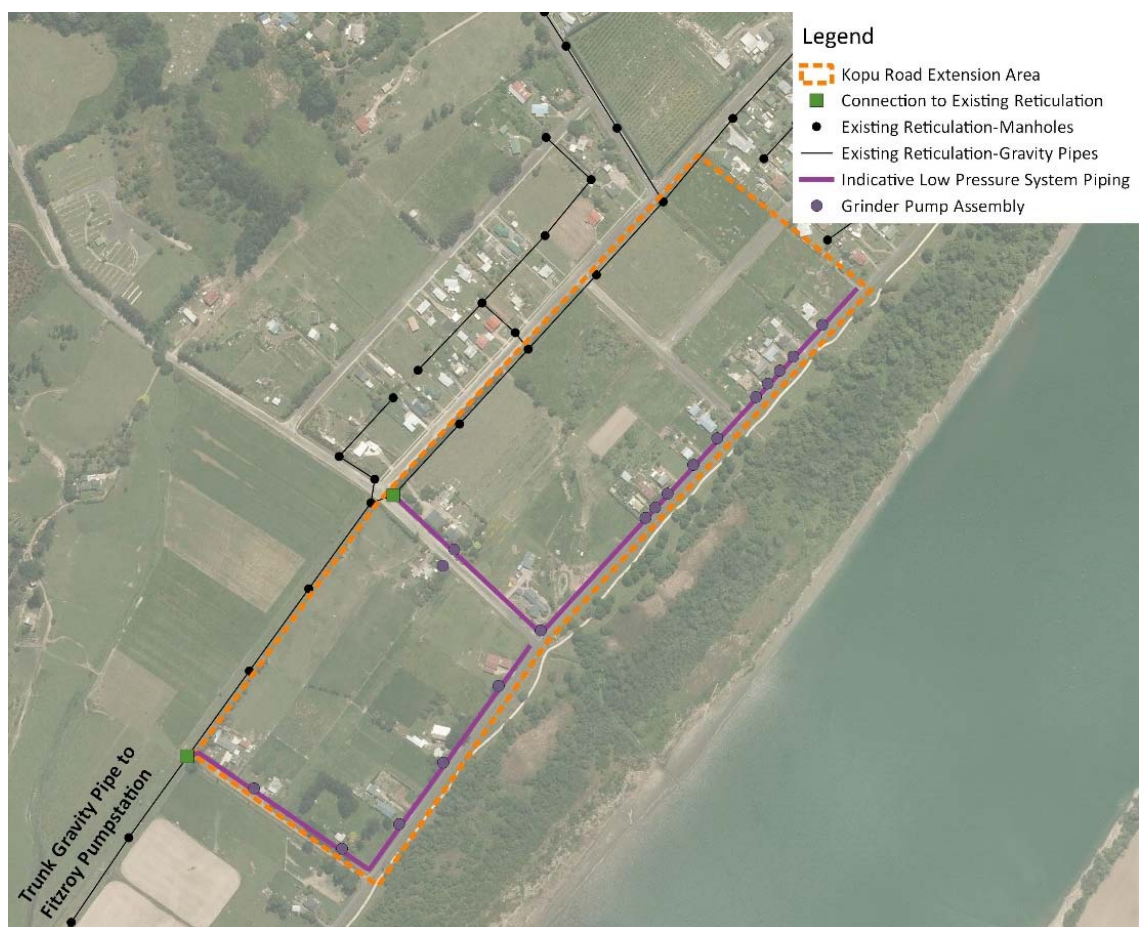
Figure 4.16 Kopu Road Extension Area - Low Pressure Sewage System
