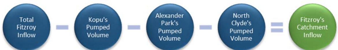
Figure 3.5 Calculation of Fitzroy Pumpstation's Associated Catchment Inflow
